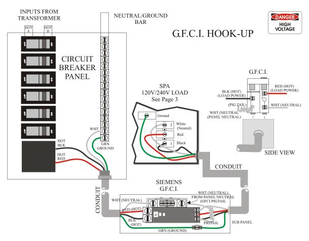
An illustration showing the proper electrical connections for 240 volt service has been provided for you on a wiring diagram and conversion instruction affixed to the backside of the electrical box faceplate. Be sure to follow these and all other instructions carefully. Be sure that all connections are tight before switching on the circuit breaker.
